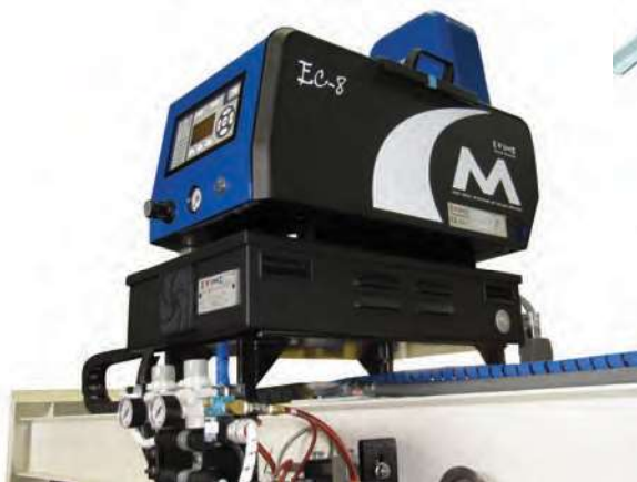
Hotmelt and Cold Set Glue Units
