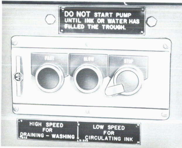
FIGURE 4-7. INK CIRCULATING PUMP PANEL
